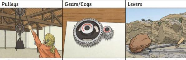
Pulleys can be used to make a small force lift a heavier load. The more wheels in a pulley, the less force is needed to lift a weight. Gears or cogs can be used to change the speed, force or direction of a motion. When two gears are connected, they always turn in the opposite direction to each other.
